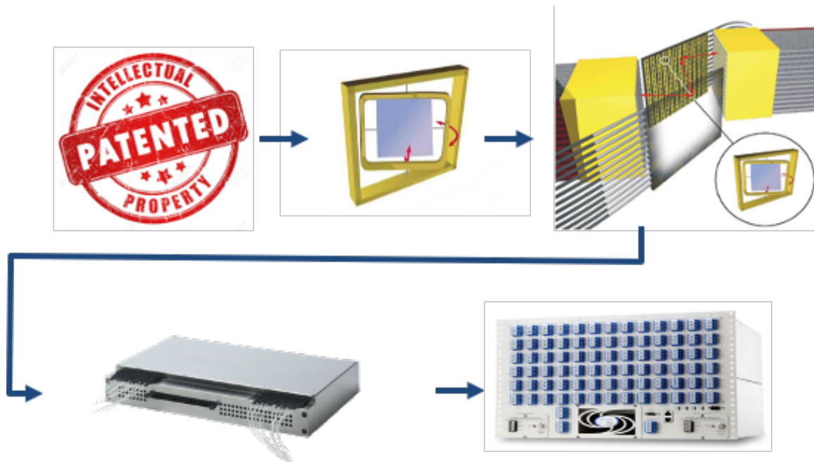
An optical switch tech stack: IP, component, module, subsystem, and full system. (Based on Calient's 3D MEMS innovation.)
